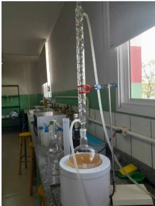
Figure 5: Laboratory Setup for Ethanol Distillation Using a Fractional Distillation Column
