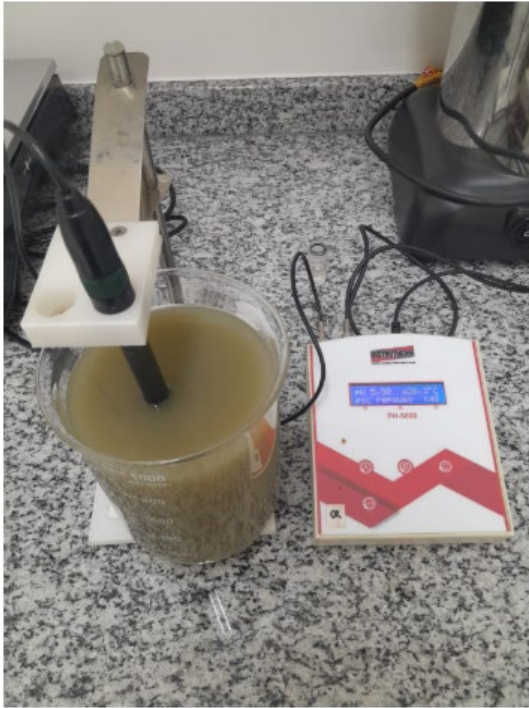
Figure 4: pH Measurement of Fermentation: Biofuel Production Process from Sweet Potatoes
